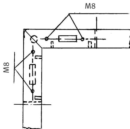
2. Lay upper net hoop fixing angle on bar/upright construction (so that bore holes of the angle are situated upon those of the bar/upright construction) and fix them with 4 safety hexagonal socket screws M 8x50 each .
