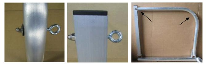
Stick ring nuts M 6 x 50 through boreholes of the net hoop (position see picture below) and fix them with washer DIN 9021, 7.4 x 22 and self-locking cap nut DIN 986, M 6. Take care that rings point to the inside.
