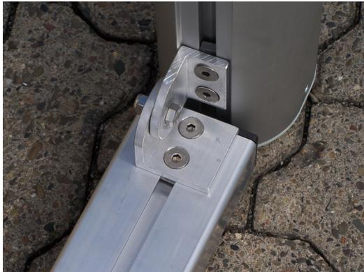
7. Adjust ground frame and tighten screws mentioned in position 5.
