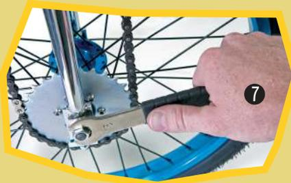
Finally, tighten the axle-screws equally and step by step on both sides to fix the wheel in the frame. (7)
