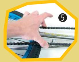
Next, tighten the 10mm nuts to adjust chain-tension. It should be tight enough, for being able to push the chain around 5 mm together with your hands when grabbing like on (5). Tighten both sides equally and step by step to make sure the wheel is in the middle of the frame like shown on (6).
