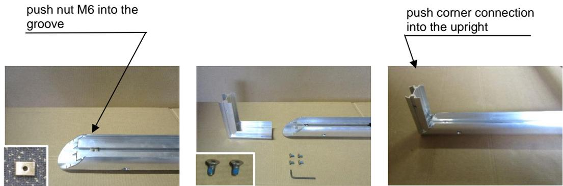
Stick open ends of frame on both corner connections und screw 2 safety hexagon socket screws each DIN 7991, M8 x 16 (see picture bottom right). Adjust Corners and tighten all screws.
