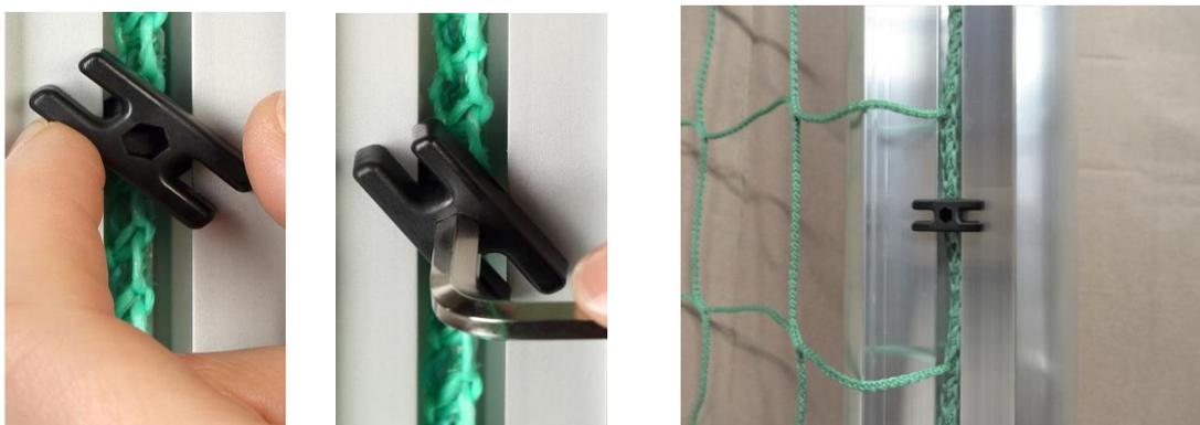
Pull the cord through each net meshes and fix it on both net hoops, if necessary lead it through the bore in the net hoop.
