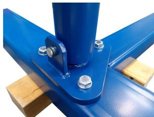
Position a large pillar on the raised threshold according to the hole pattern and hold the pillar firmly. Fix the column by tightening the screws with a 19 mm socket and a 19 mm key.
