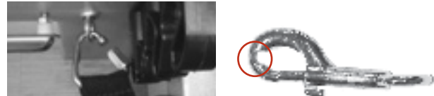
Figure 2: Good snap: no wear on hook. Bad snap: excessive wear on hook.
