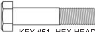
KEY #51 HEX HEAD BOLT 3/8" X 1 3/4" PARTIAL THREAD QTY. 22
