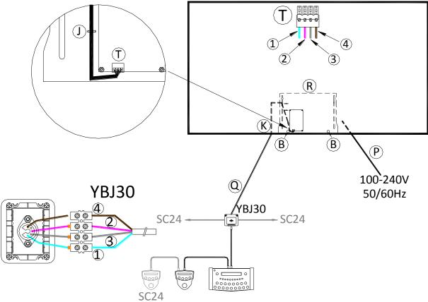
Control cable (Q): (1) = GND = blue wire / (2) = Rx + = white wire / (3) = Rx - = grey wire / (4) = +24V = transparent wire
