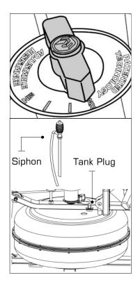
Row a minimum of ten complete strokes before commencing tank draining. Remove tank plug, insert rigid end of siphon into tank and begin draining.
