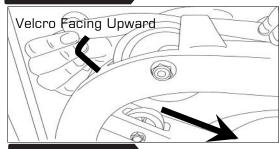
Begin reattaching the Rower Belt by threading around the Rower Belt Pulley with the Velcro side facing upward as illustrated.
