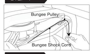
Rethread the Bungee Shock Cord (on opposite side of the Idle Wheel) back through the Bungee Pulleys and tie off at the Attachment Point.
