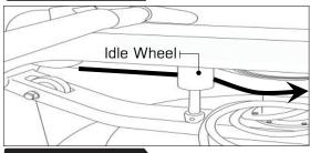
Next, thread the Belt around the Idle Wheel as shown. Once around the Idle Wheel, attach the Rower Belt to the Belt/Bungee Pulley. There is an obvious "lip" at the attachment point.
