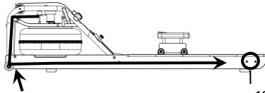
**Hint:** Before reattaching the Inner Clip/ Bungee Hook, tie a slip knot under slight tension at the lower bungee pulley. This will keep the bungee under tension while reassembling the Bungee Hook.
