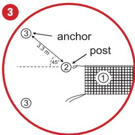
**3** To obtain the ideal position for the sand anchors, unfold the net completely **1**. The loops at the ends of the top cable mark the places for the posts **2**. Drive the anchors into the ground at a distance of approx. 3.3 m from the post position to form an angle of approx. 45deg with the post **3**. Please refer to figure 7 at the bottom of this page to get an overview of the correct placement of posts and anchors.
