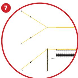
**7** The net tension and net height can be altered to achieve the perfect net by adjusting the straps and the tension of the ropes at the bottom corners of the net.
