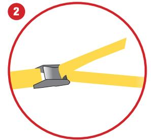
**2** Assemble the two parts of the yellow straps as shown. Make sure the loops are positioned at the ends of the belt and not near the metal clip lock. Place the small loops of the straps under the disks on the top of the four sand anchors.
