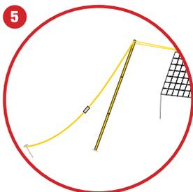
**5** Put the loops on the other end of the straps over the top end of the posts and put the posts up sloping inwards. Then position the cable loops attached to the top ends of the net over the top of the posts as well.
