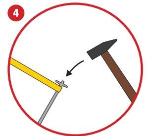
**4** Use two anchors per post. Make sure to knock the anchors into the ground at a slight angle away from the posts to aid tensioning.
