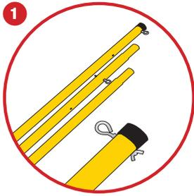
**1** Each post is assembled from three pieces. The section with the black cap is the top piece. Insert the metal eyebolts into the holes and secure with the threaded nut provided. You can choose between the two different holes to obtain different net heights.
