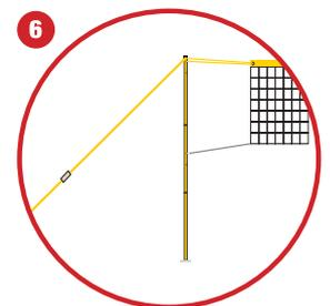
**6** Tighten the yellow straps and adjust the position of the post as necessary to get the posts upright. The net must be aligned midway between the poles by adjusting the short yellow ropes at the top of the net. Adjust the lower ropes to length at the metal eyebolts at the poles.
