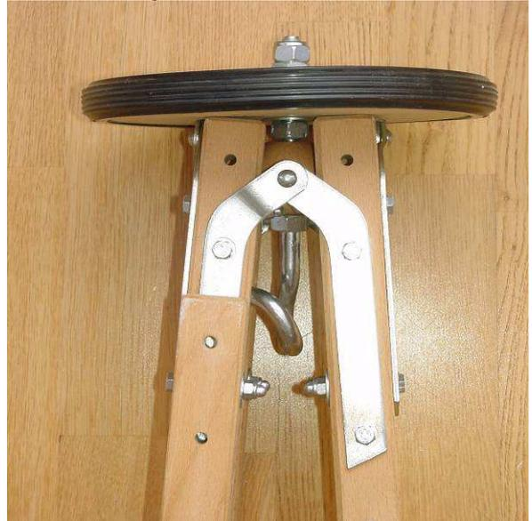
Step 3 and 5: Setting up and assembly of stabilisation cross bars.
