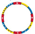
The Spectra System  $^{\text{TM}}$  consists of coloured reference points and dots on the capsule that are easy and quick to read and memorize.
