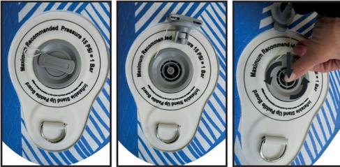
Make sure that the valve is free of sand or dirt. Unscrew the valve cap. Slowly press down the button on the valve to start letting the air out of the board. There will be an initial burst of air, but that will slow down quickly. Push button in and turn it clockwise to the right, and lock into „DOWN“ position.
