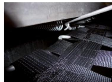
Hinging or unhinging the steel springs with the mounting tool
