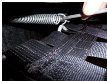
Hinging or unhinging the steel springs with the mounting tool
