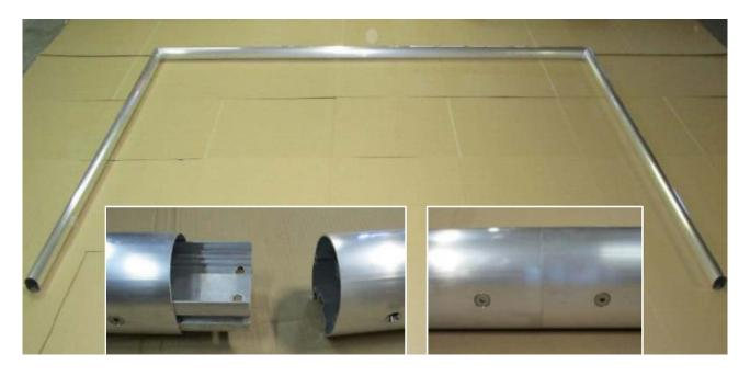
b) Turn the complete goal frame so that the guide rail faces upwards. Place net hoops in the upper corners and at uprights above threaded holes in the guide rail and screw safety hexagon socket cylinder screws DIN 912, M 6 x 20 together with washers DIN 9021, 7.4 x 22 mm.
