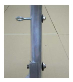
d) Stick from the inside ring nuts M6 x 50 for tensioning net rope through the open boreholes of both net hoops and fix with washers DIN 9021, 7.4 x 22mm and nuts DIN 985, M6.
