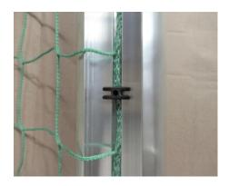
Pull the cord through each net meshes and fix it on both net hoops, if necessary lead it through the bore in the net hoop.
