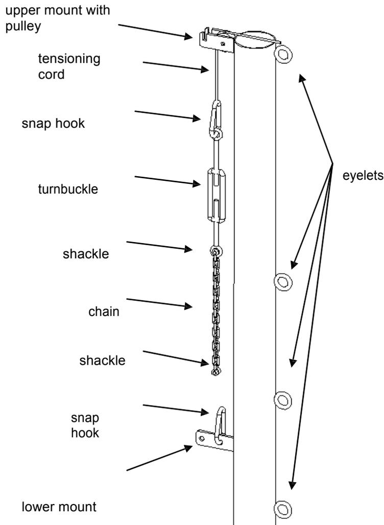
**Illustration 3: tensioning mechanism**
