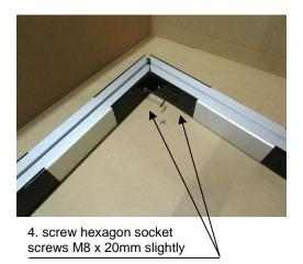
Then join uprights at the external corner. Adjust crossbar and uprights. Screw 2 hexagon socket screws DIN 7991, M8 x 20mm in the external corner (see picture bottom right) and tighten all screws.
