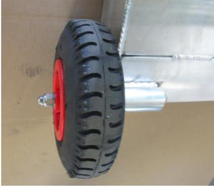
3. Stick the wheel on the round tube and then add another washer DIN 125, Ø 13mm. Now screw and tighten self-locking nut DIN 986, M12.
