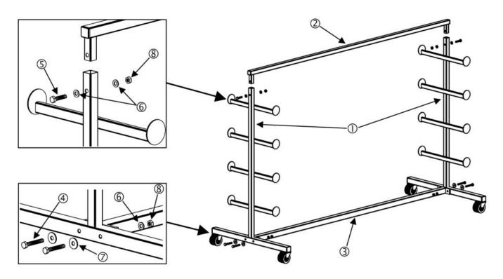
To assemble the transport trolley, insert the strut with plug-in tubes ② into the two side sections ① from above.
