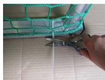
c) Fix net at the bottom of net hoops with 3 cable clips.Cut projecting parts.
