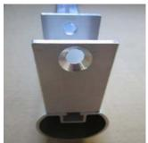
c) To fix the lower hinge stick from the bottom (upright's end) 1 nut 20 mm, M 8 each in the guide rail of the upright. Mount lower hinge with 1 fastening borehole. Please consider that the inclined side of the hinge points to the goal inside. Push nut 20 mm, M 8 below the borehole of the hinge and fix it at the upright with safety hexagon socket screw DIN 7991, M 8 x 16.
