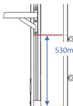
2. Fasten the tube 35 x 2 mm with 3 screws M 8 x 20mm between the floaters.
