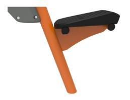
The seat is made of a Polyurethane Rubber and has a steel insert plate which connects it to the steel frame. The seat is positioned under a 12 degree angle, accommodating seating heights from 550-620mm.
