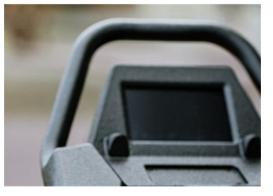
The handle bars is designed with multiple hand positions to accommodate different postures and riding styles. It is a casted Aluminium part with Polyurea coating for good grip and insulation.
