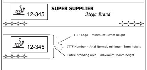
It is possible to equip the covering with two branding areas, positioned at 90 degrees to each other, but when mounted on the blade, only the one close to the handle is accepted.
